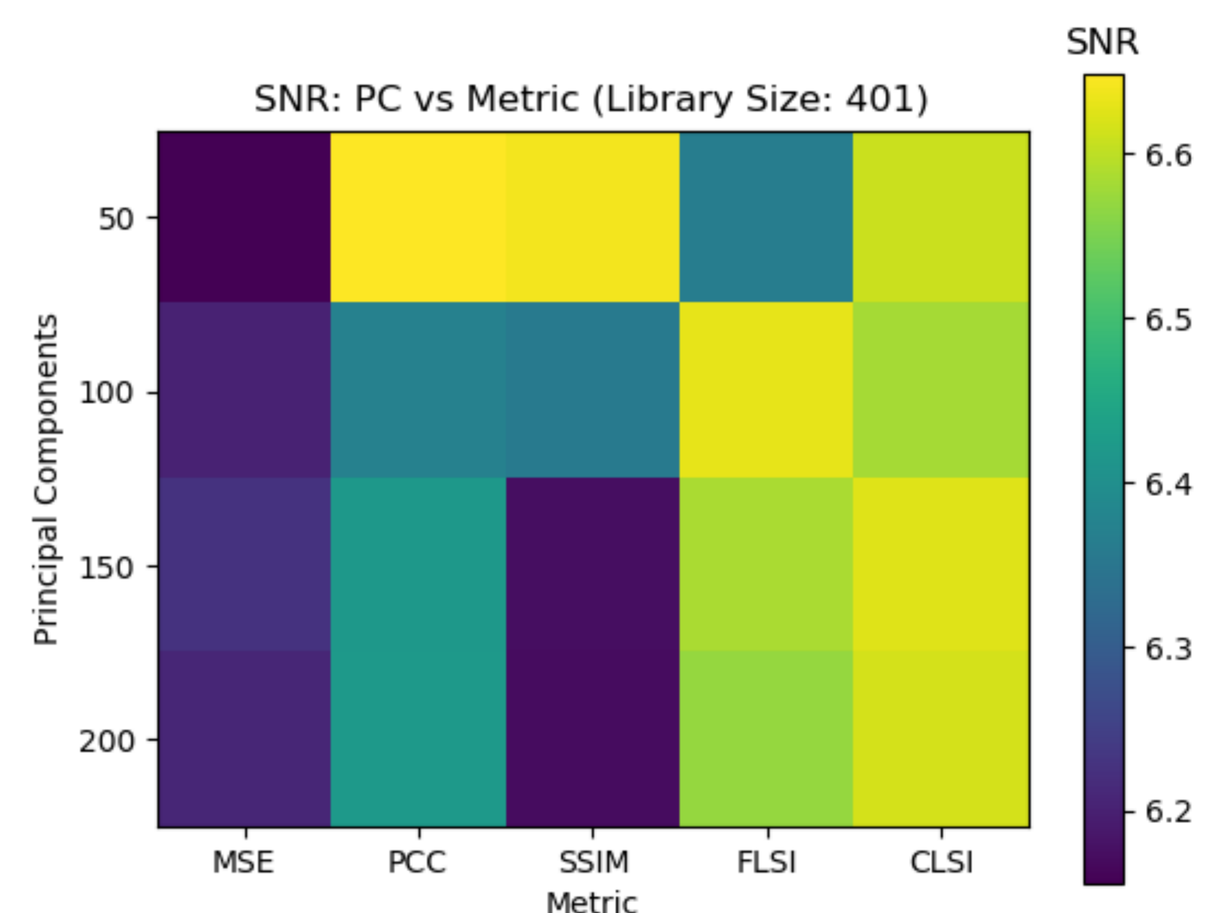
Fig 4: S/N ratio from Super-RDI reductions for HBC359 (2017/09/28), with 401 reference library size, varying similarity metrics and principal components
